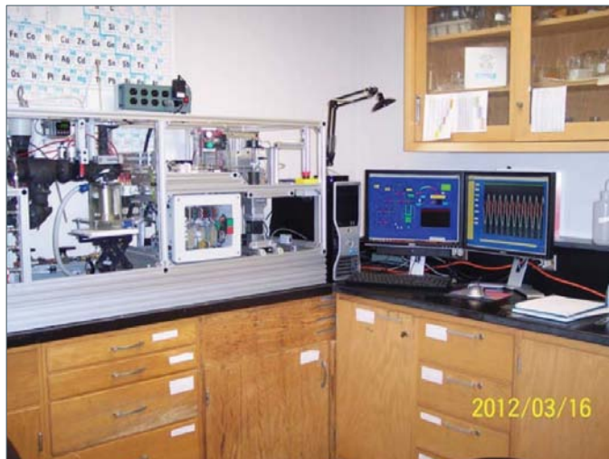
Figure 3: Photograph of Dynamic Volumetric Frequency Response (DVFR) Apparatus
