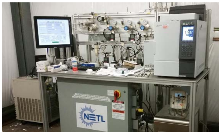
Figure 1: Hollow fiber MMMs are being fabricated and tested for their long term performance characteristics in the presence of humidity and contaminants using this test setup.
