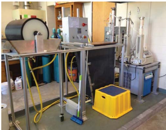
Figure 2: Georgia Tech Hollow Fiber Fabrication Line
