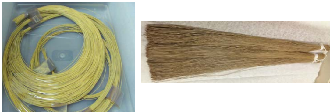
Figure 2: Photographs of Bundles of PBI Asymmetric Hollow Fibers as Spun (left) and Post Treated (right)
